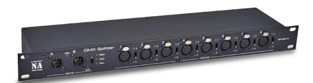
DMX Splitter 8 is used for DMX signal amplification, isolation and splitting to multiple outputs. Splitter has 2 optically isolated RDM/ DMX inputs and 8 optically isolated outputs. Each of 8 outputs can be switched to any of 2 inputs, which means that the splitter can operate as one single universe with 8 outputs or, it can be configured as two seperate splitters.
