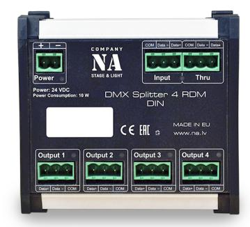
Optically isolated DIN rail mount DMX Splitter 4 is used for DMX signal amplification, isolation and splitting to multiple outputs. Splitter has one DMX input and four outputs. Avaliable in configuration with RDM. Pluggable Terminal Block (PTB) screw terminals for bare-wire, installation flexibility.
